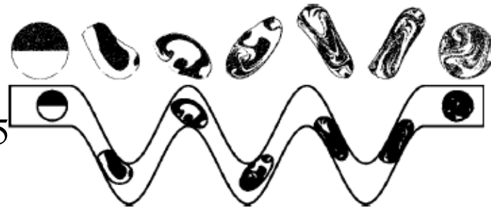
FIG. 3. Snapshots of mixing patterns taken at the nondimensional times from left to right t^*=0, 0.42, 0.90, 2.32, 1.80, 2.22 and 2.64 , respectively. The top plots are the enlarged versions of the corresponding scatter plots shown in the channel (bottom plots). ( Ca=0.025, Re=6.6, \lambda=1.0, \Lambda=0.76 , Grid: 1024 \times 64 .)
