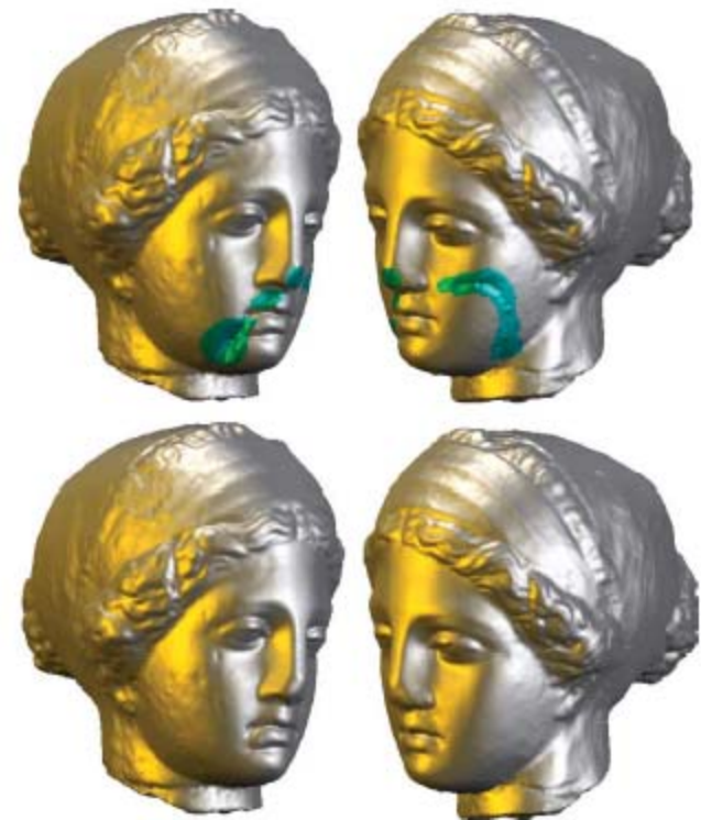
Fig. 3. Initial (top) and restored surface (bottom) of a venus head dataset from two different views. The areas of the surface to be restored are shown in darker grey. The time step was chosen as \tau = 10^{-6} , the restored surface corresponds to time T = 20\tau and the grid size of the initial mesh varied between 0.0013 and 0.012. The initial object was scaled to diameter 1.
