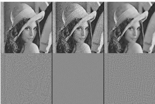
Fig. 4 The Lena image with 20% Gaussian noise added is denoised three ways. First row (left to right): “2nd Order”, denoised with (1.1); “4th Order (1)”, denoised with (2.7) for a short time; and “4th Order (2)”, denoised with (2.7) for a long time. Second row: the method noise for each image. The initial clean and noisy images are the same as in figure 2
