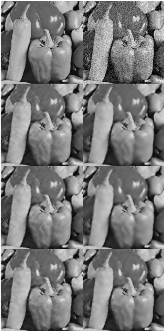
Fig. 7 Peppers with 20% Gaussian noise denoised with (2.7) (second row), (4.1) (third row), and (4.2) (fourth row), at two different stopping times. The initial clean and noisy images are shown in the first row.
