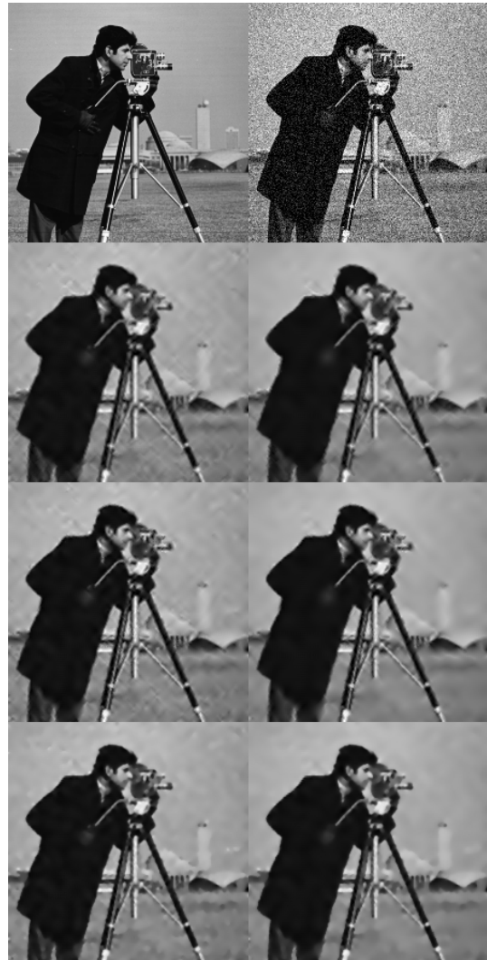
Fig. 6 Cameraman with 20% Gaussian noise denoised with (2.7) (second row), (4.1) (third row), and (4.2) (fourth row), at two different stopping times. The initial clean and noisy images are shown in the first row.
