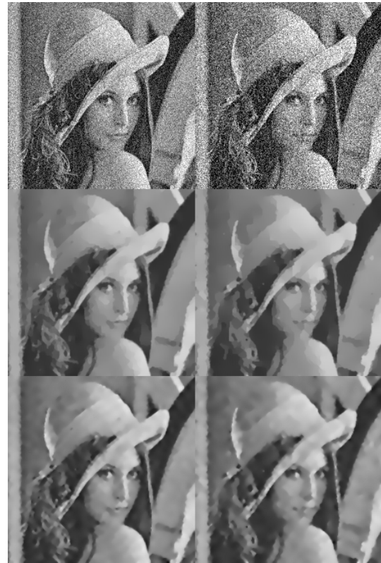
Fig. 9 Denoising results using (2.3) and (4.2) on an image with 20% (left column) and 30% (right column) Gaussian noise. First row: initial noisy images. Second row: results denoising with (2.3). Third row: results denoising with (4.2). The initial clean image can be seen in figure 2.
