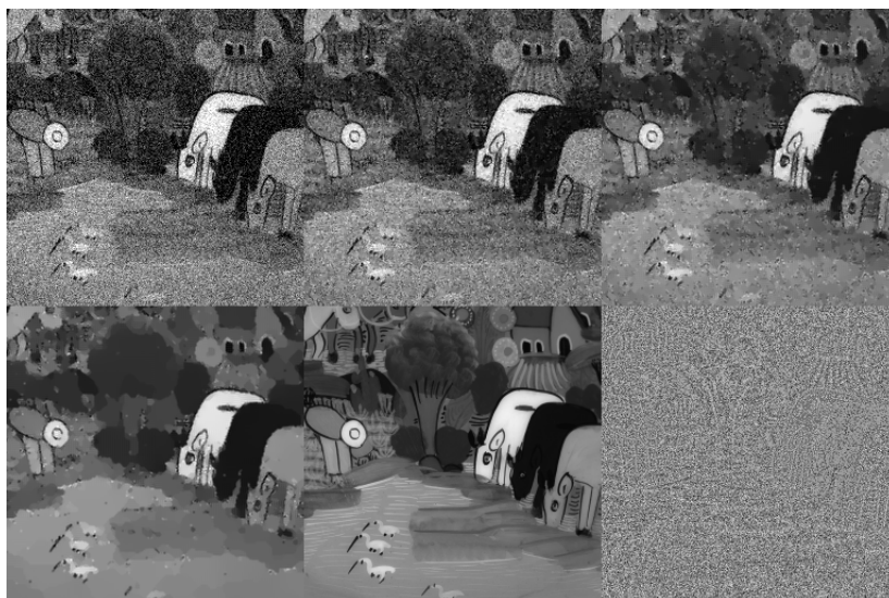
FIGURE 13. An experiment with intense noise. SNR is 1.59 and PSNR goes from 18.84 to 26.70.
